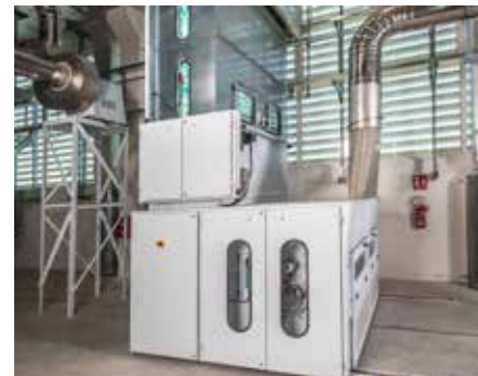
The fine opener TBL-FO for natural fiber processing
