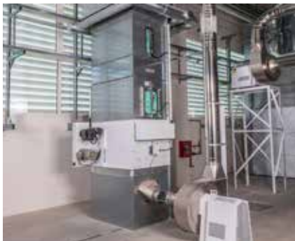
Feed box TBL-FB for fine opening in man-made fiber lines
