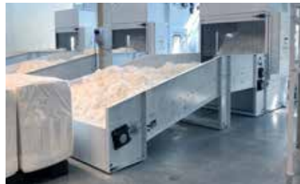
Bale opener TBL-BO is adjustable to a wide range of fibers
